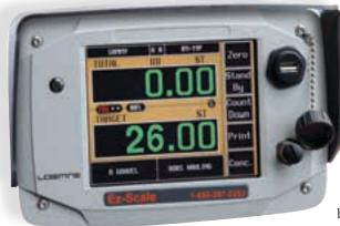
Newer in-cab display devices use touch screens instead of push-buttons to control the features. They offer higher resolutions and adjustable brightness, which is helpful when switching between indoor and outdoor operations. The port for transferring data into a USB flash drive is on the front of this device; some companies also offer Wi-Fi or Bluetooth data transfers.
